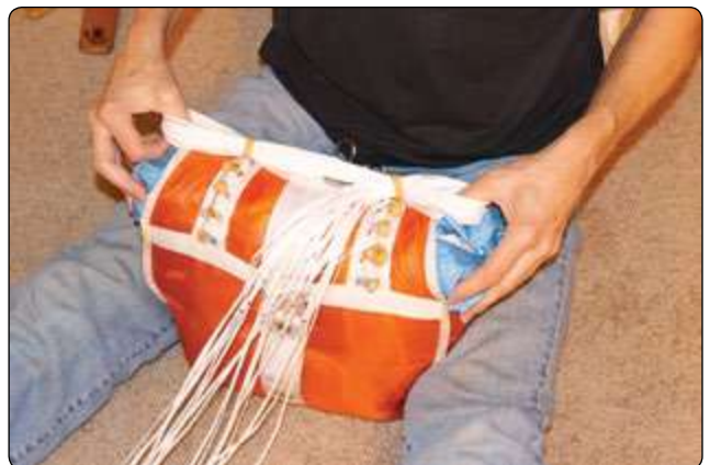
Figure 5-140. Stow the lines from top to bottom. Each stow is a locking stow.
