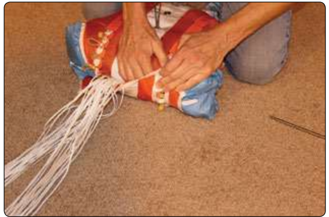
Figure 5-139. The top flap closes first so that the rubber bands come through the slots in the bottom flap.
