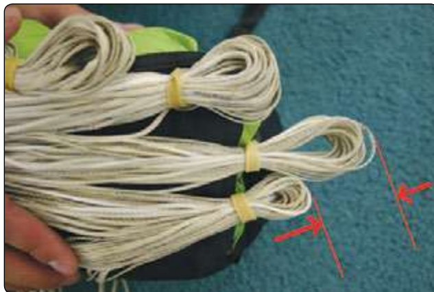
Figure 4-39. Line stow length comparison.
