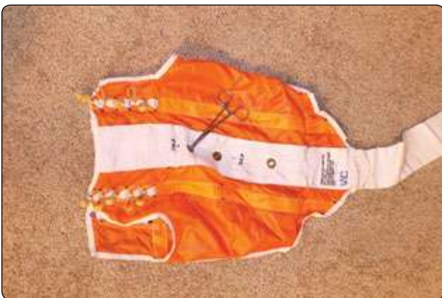
Figure 5-134. Prepare the Reserve Deployment Speed Bag by using a hemostat to pinch the inner buffer tabs together as shown.
