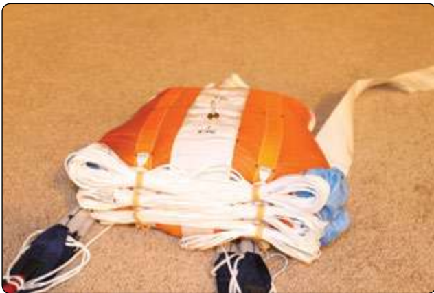
Figure 5-142. Insert a bodkin through the channel in the bag where the hemostats were.
