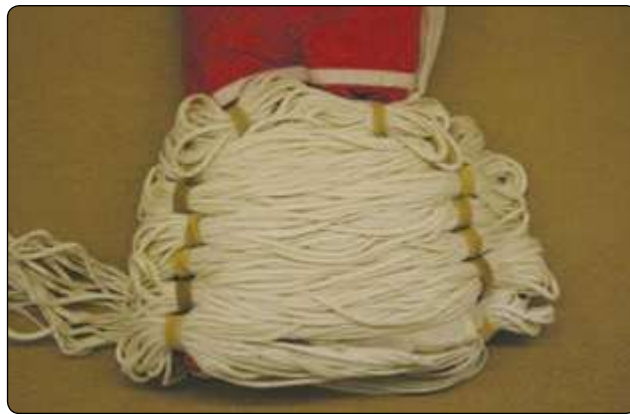
Figure 2-23. Type 3 deployment—Phantom canopy.
