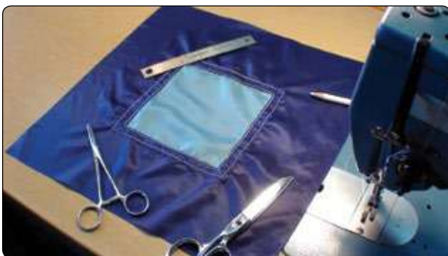
Figure 7-28. Correct stitch gauge.
