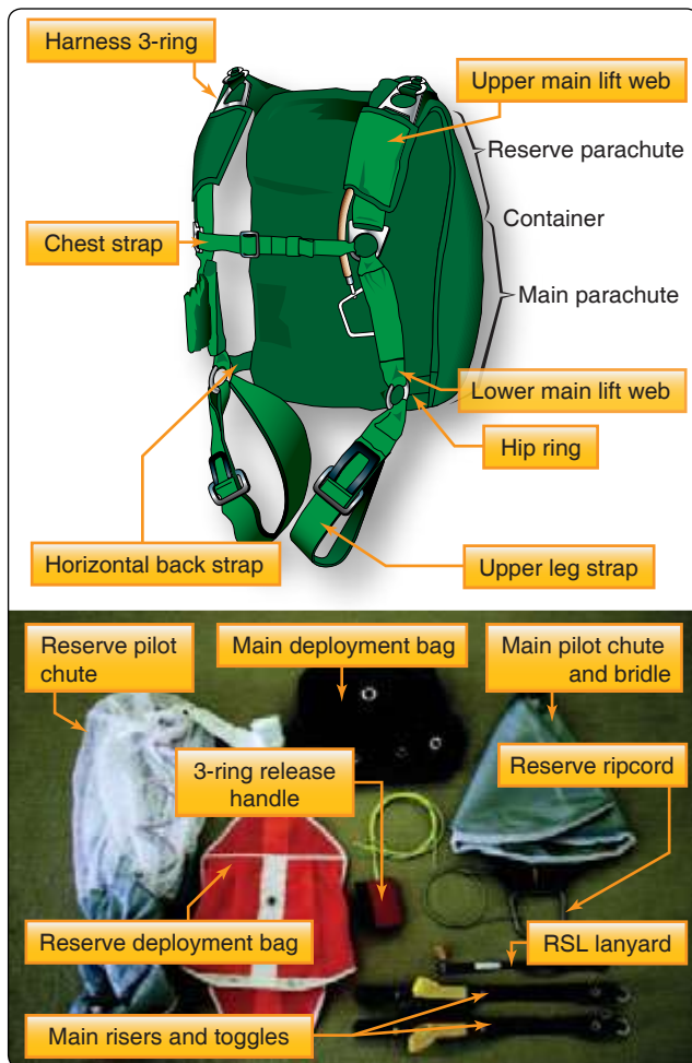
Figure 2-2. Subcomponents of the harness/container assembly.
