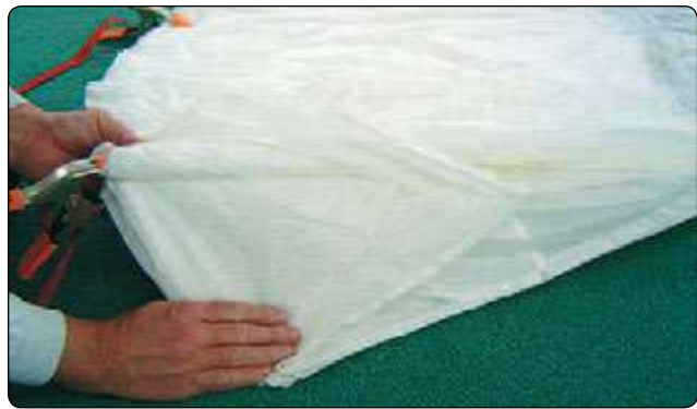
Figure 5-76. Fold half under "A" lines.
