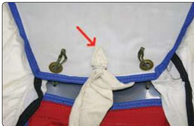
Figure 2-11. Square reserve hesitator loop configuration.
