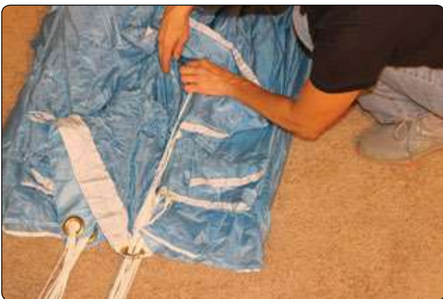
Figure 5-123. Pull the lines taut and to the center.
