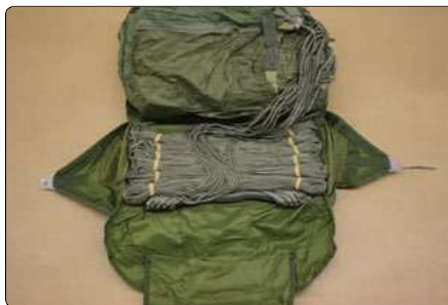
Figure 2-21. Type 1 deployment—T-7A reserve.
