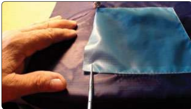
Figure 7-21. Correct patch tension.
