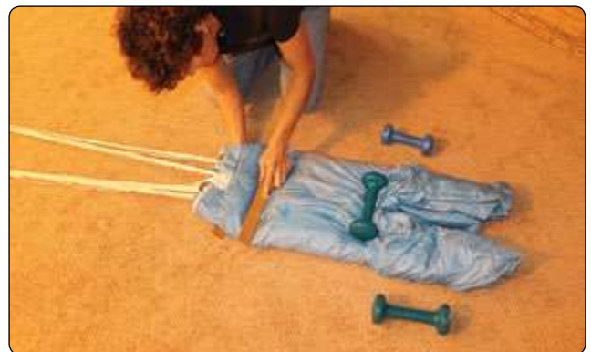
Figure 5-131. Two packing paddles can be used to make a neat S-fold.
