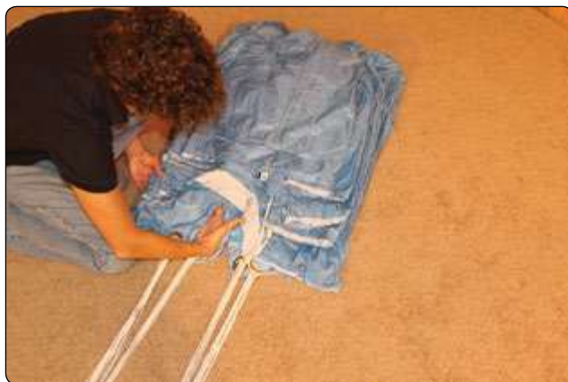
Figure 5-126. Tuck the slider up between A/B and C/D line groups. Some manufacturers recommend stowing the apex of the slider with a rubber band to the center B or C line attachment tab (whichever one it best aligns with).
