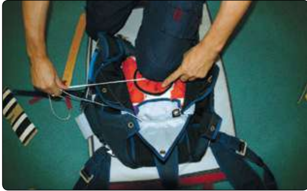
Figure 5-109. Position pilot chute.
