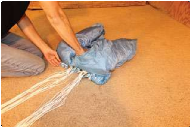
Figure 5-133. Make a second S-fold with the upper part of the canopy on top of the lower part.
