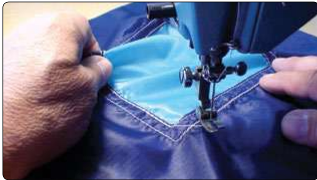
Figure 7-33. Always grab the work by the threads and remove directly to the rear when removing it from the machine to avoid bunching.
