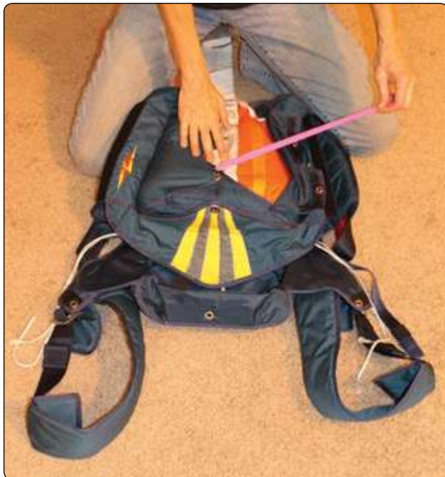
Figure 5-149. Close either side flap (not side-sensitive).
