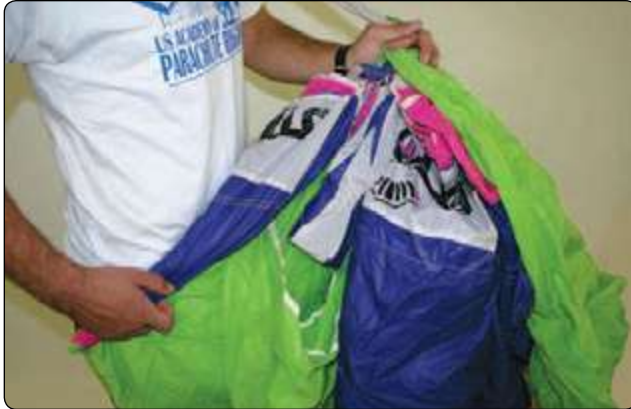
Figure 4-36. Rolling the nose of the canopy.
