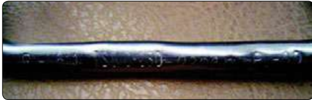
Figure 5-3. Reserve ripcord with TSO markings.
