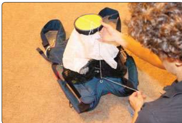
Figure 5-157. Thread pull-up cords through each closing loop and through bodkin eyes.
