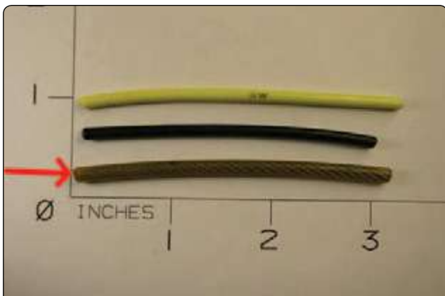
Figure 3-101. 7x7 stainless steel corrosion resistant cable.
