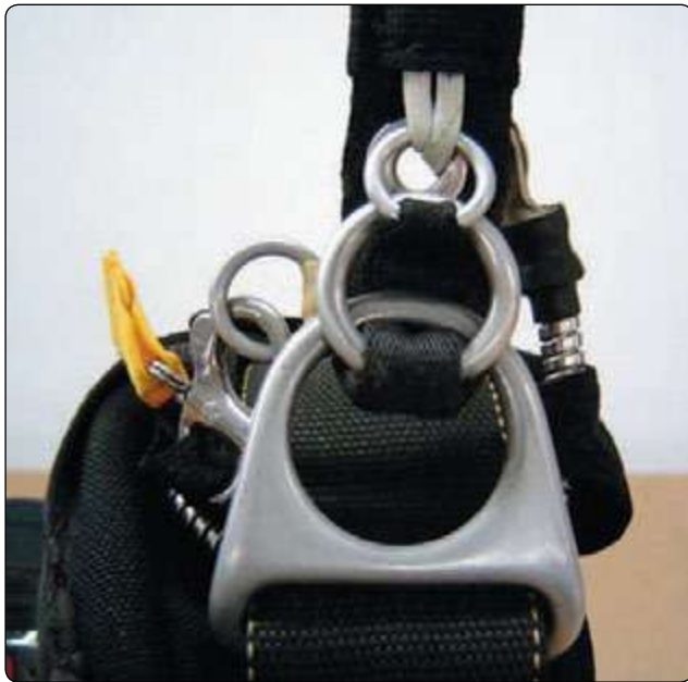
Figure 5-26. 3-Ring ® release system.
