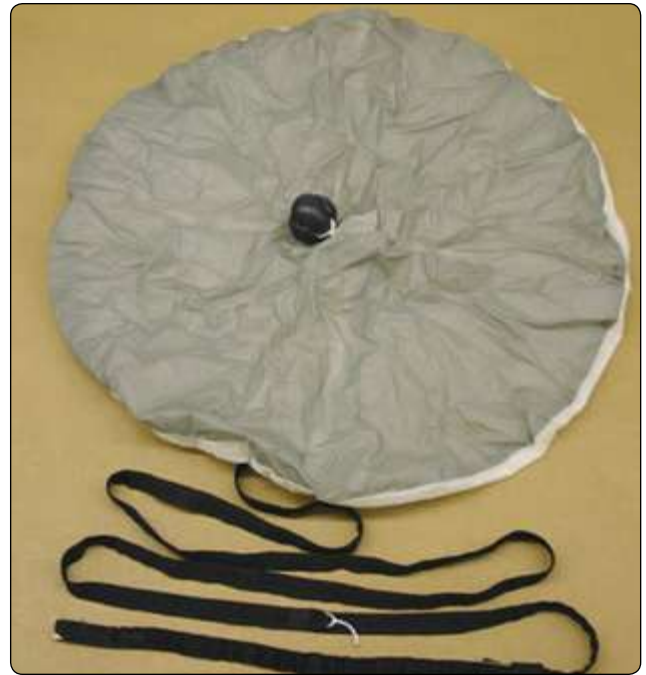
Figure 2-42. TOP bridle/pin configuration.
