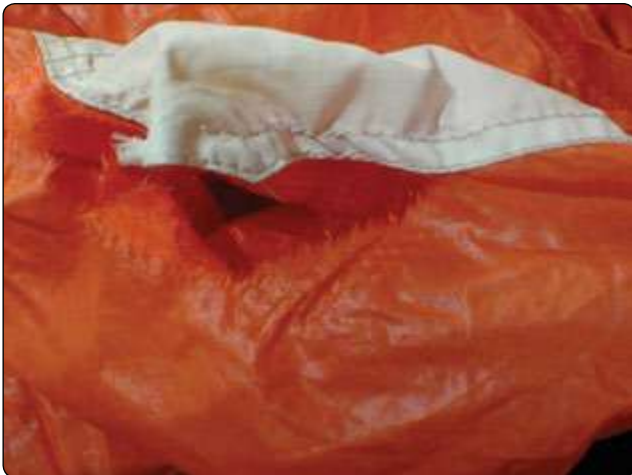
Figure 7-11. Pilot chute attachment damage is not always obvious.
