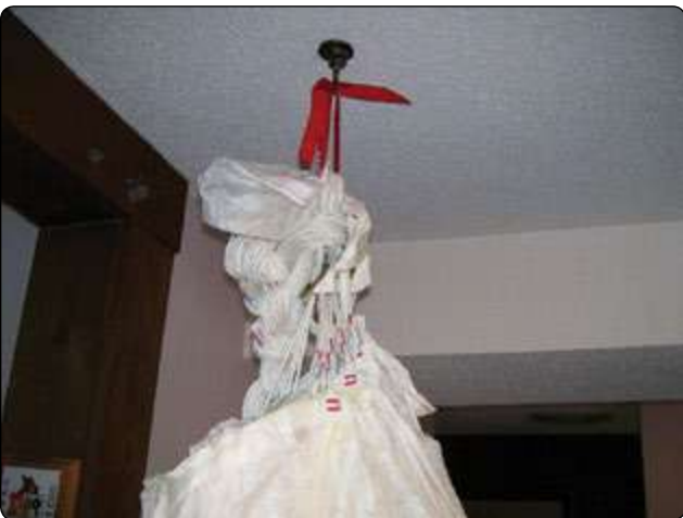
Figure 6-89. A square canopy can also be aired by S folding and hanging it from a simple hook.
