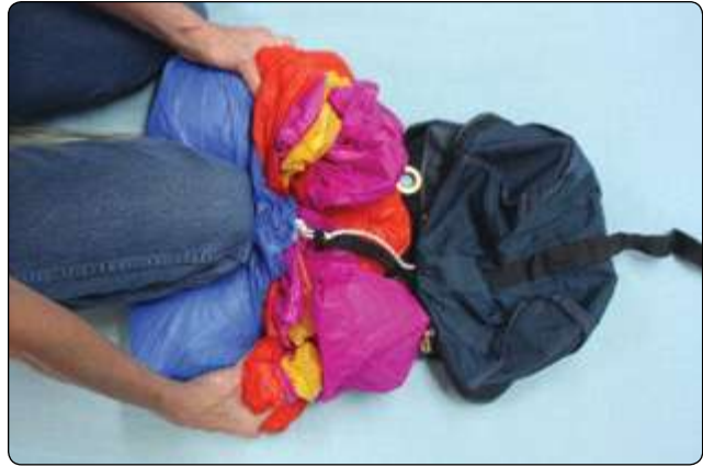
Figure 4-24. Most canopies take two S folds. Pull PCA ring outward so that it is up against the grommet inside the bag.
