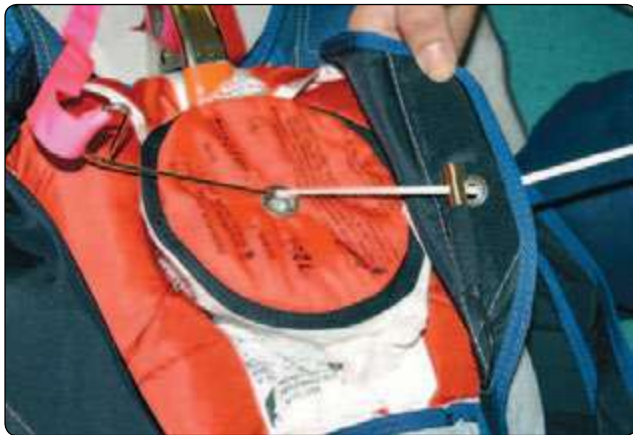
Figure 5-110. Route pull-up cord through cutter and right flap.
