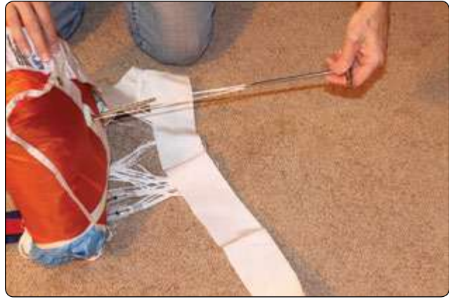
Figure 5-144. The second bodkin is now threaded through the bag in the opposite direction.
