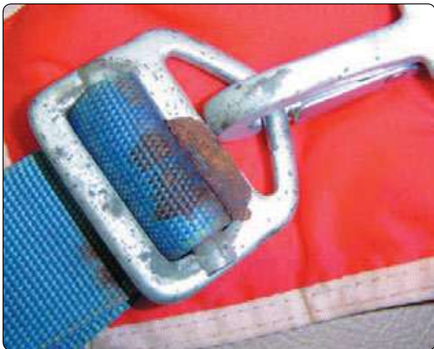
Figure 5-17. Rusty leg snap hardware.
