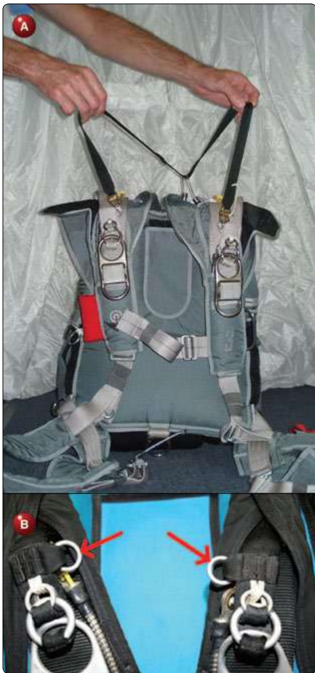
Figure 2-50. A) Dual-side RSL configuration and B) dual-RSL routing diagram.
