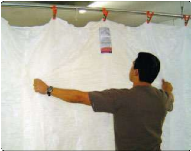
Figure 5-20. Ram-air canopy hanger—top skin inspection.
