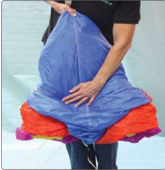
Figure 4-15. Press the air out of the canopy.
