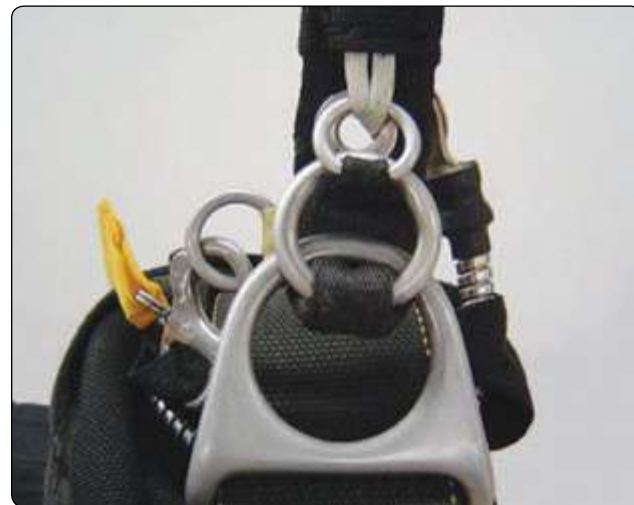
Figure 2-49. Single-side RSL configuration.
