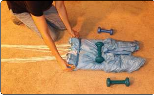
Figure 5-132. The length and width of the S-fold is determined by the width of the container and the distance between the main/reserve vertical partition and the bottom flap grommet.
