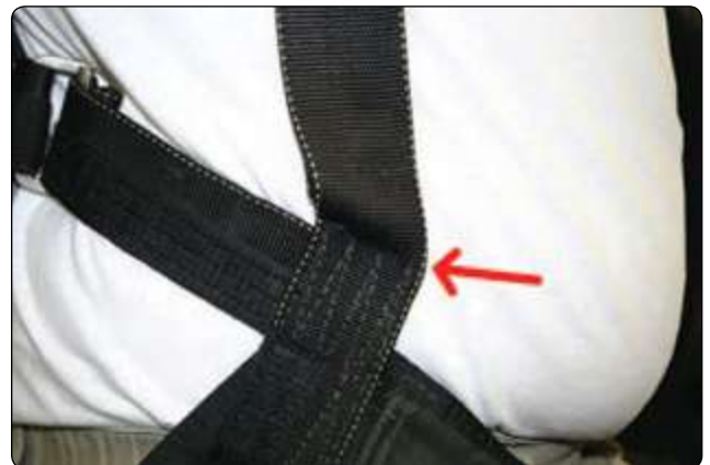
Figure 2-18. Stair-stepped harness (aka stepped harness) junction warping.
