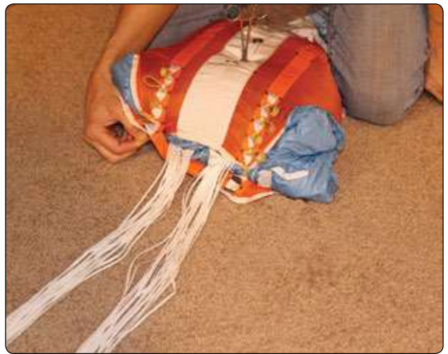
Figure 5-138. Use the flaps of the bag to control the canopy and help push it into the bag.
