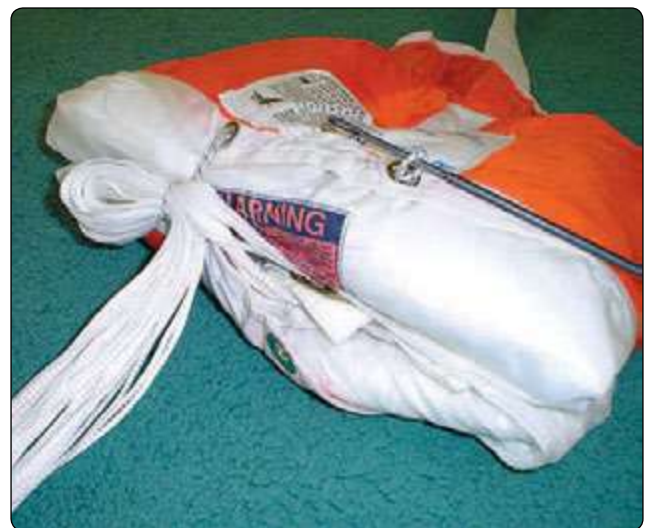
Figure 5-102. Close bag and secure locking stows.
