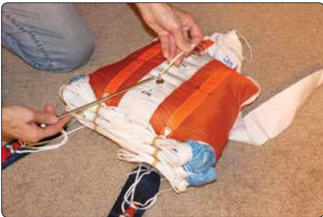
Figure 5-143. Pull a second bodkin through the bag using a pull up cord.
