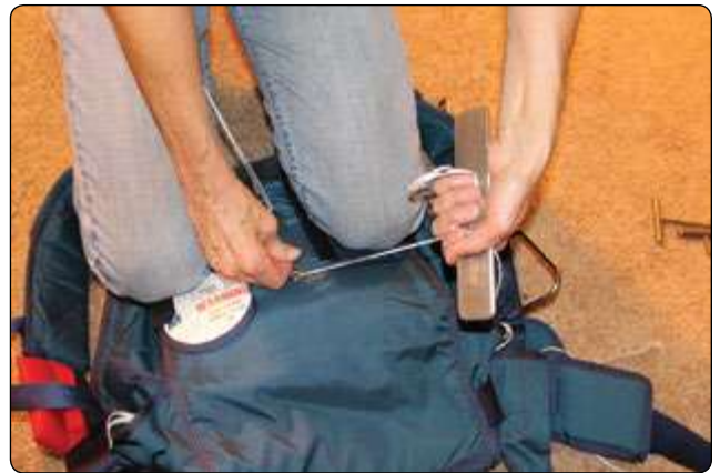
Figure 5-162. Pull bottom closing loop through the grommet and insert pin.
