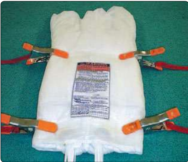
Figure 5-94. Finish wrapping tail, four clamps.
