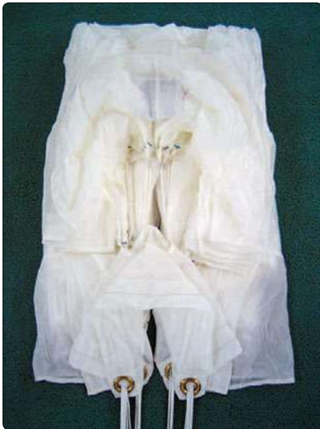
Figure 5-89. Fold tail back for wind channel.
