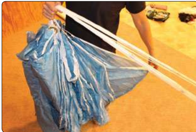
Figure 5-118. Flake the nose cells of the canopy.
