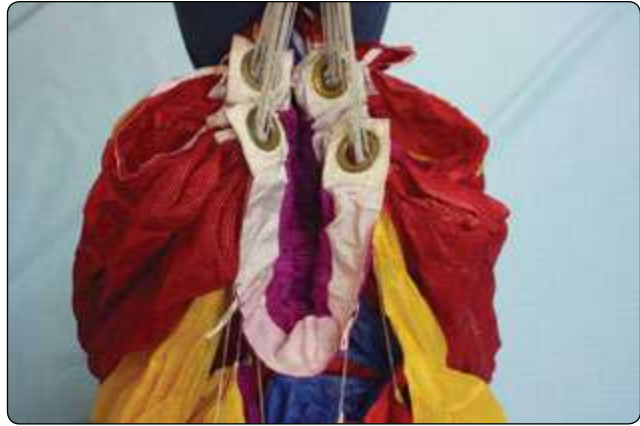
Figure 4-12. The slider can be quartered or simply halved with the slider grommets resting up against the slider stops at the stabilizers.
