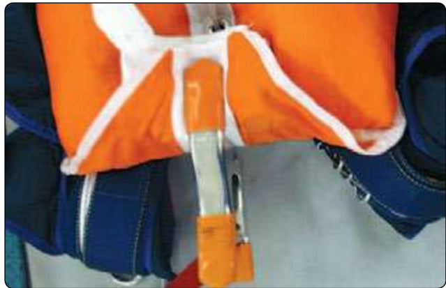
Figure 5-107. Secure yoke/bridle with clamp.
