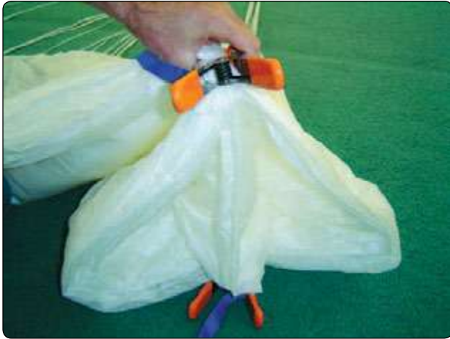
Figure 5-79. Lower “B” clamp to “A” clamp, spreading the cells.
