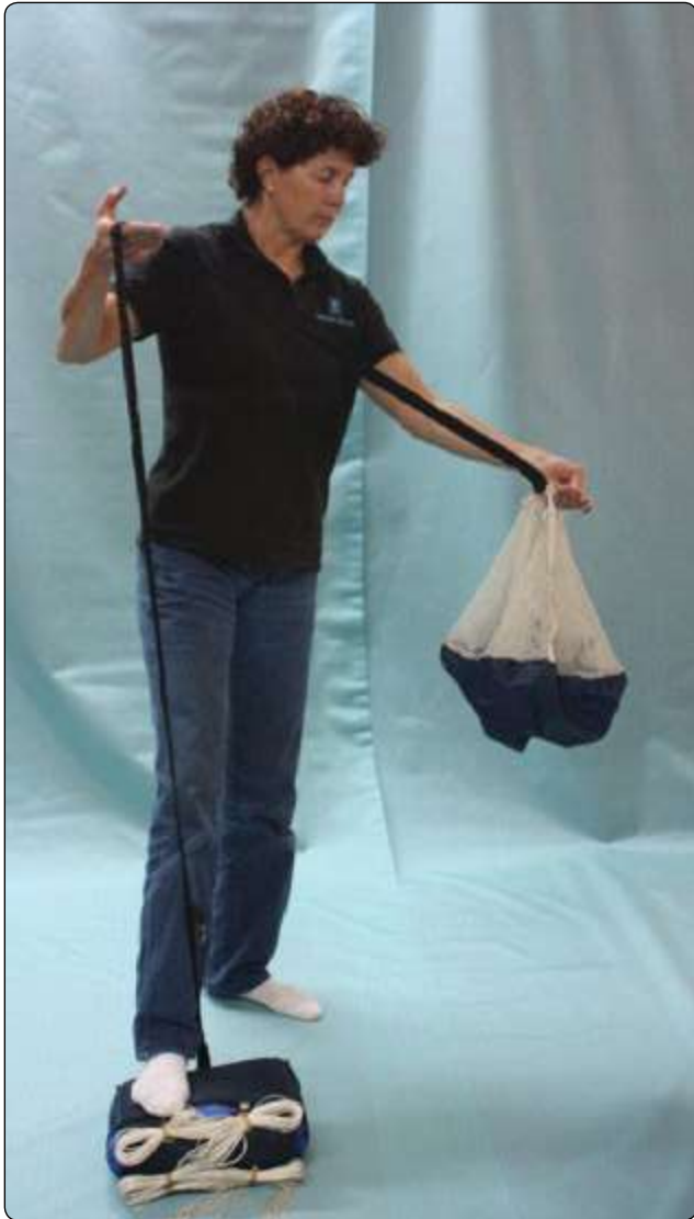
Figure 4-34. Pull the kill line through the bridle.
