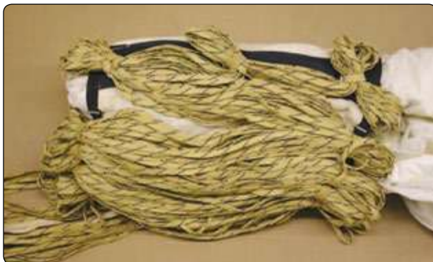
Figure 2-24. Type 4 deployment—Preserve diaper.
