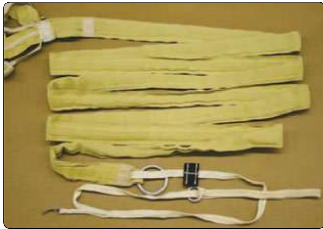
Figure 2-39. Tandem main collapsible bridle.
