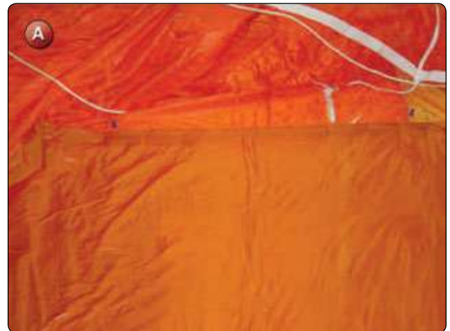
Figure 7-33. Always grab the work by the threads and remove directly to the rear when removing it from the machine to avoid bunching.
