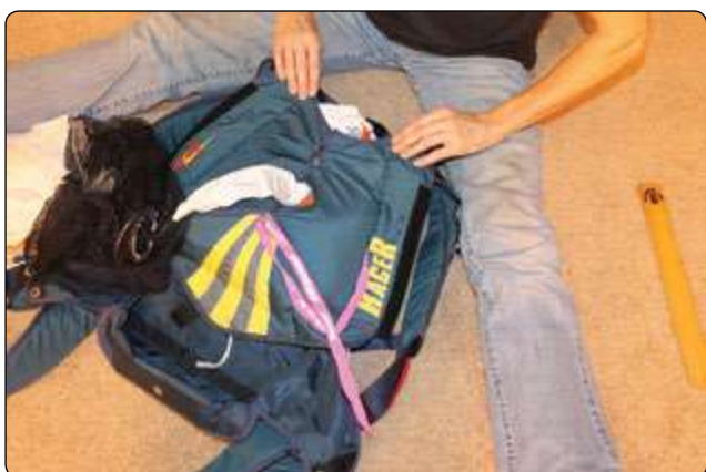
Figure 5-154. Close other side flap leaving a short section of bridle below the pilot chute.
