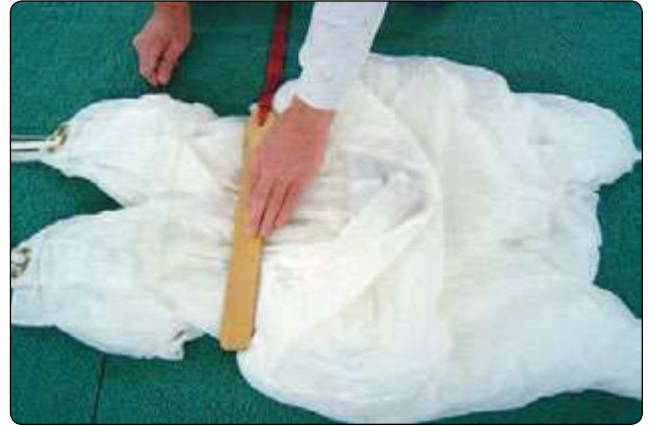
Figure 5-91. Packing paddle at \frac{1}{3} rd location.
