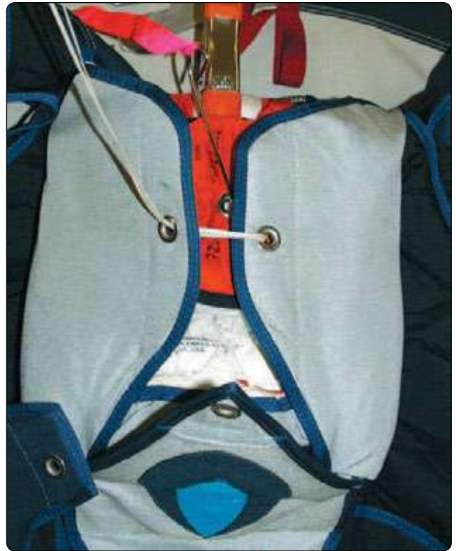
Figure 5-111. Close right and left flaps simultaneously.
