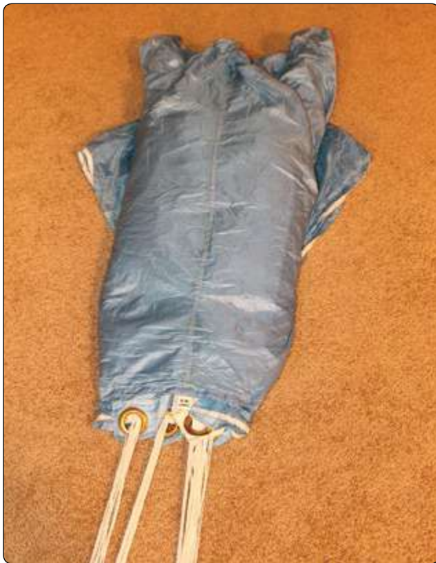
Figure 5-129. Cocoon the canopy by wrapping the tail around and under. The nose is splayed out with three cells to the right, three cells to the left, and the center cell in the middle.
