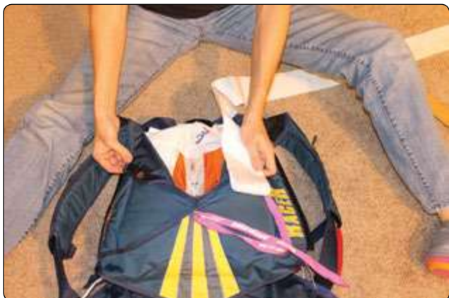
Figure 5-152. S-fold bridle and evenly distribute on both sides of container.
