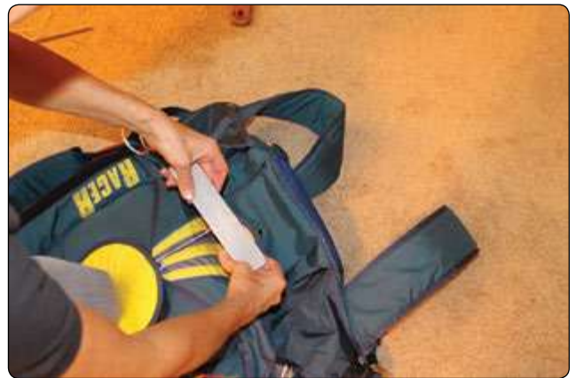
Figure 5-163. Pull on running ends of adjustable closing loop to shorten the opposite loop until pilot chute is sufficiently seated.
